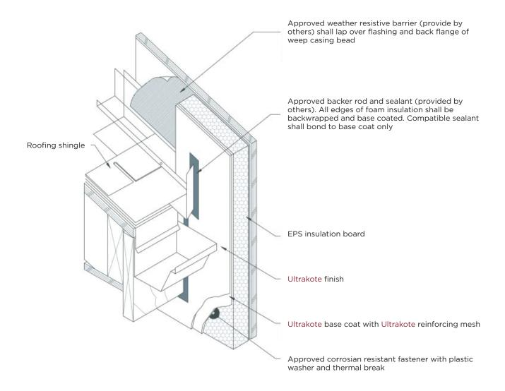
NOTE 1: Do not install the gutter system until the water managed EIFS system has been completed.
